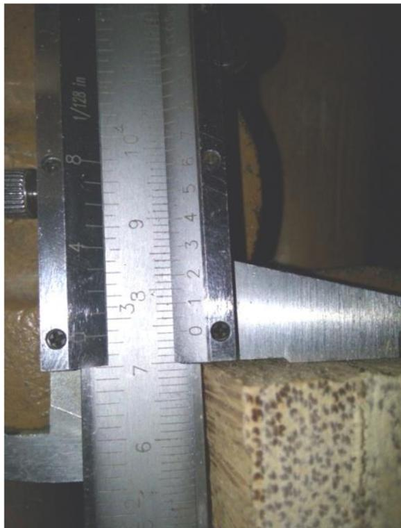
**Fig. 7** Tangential swelling test
