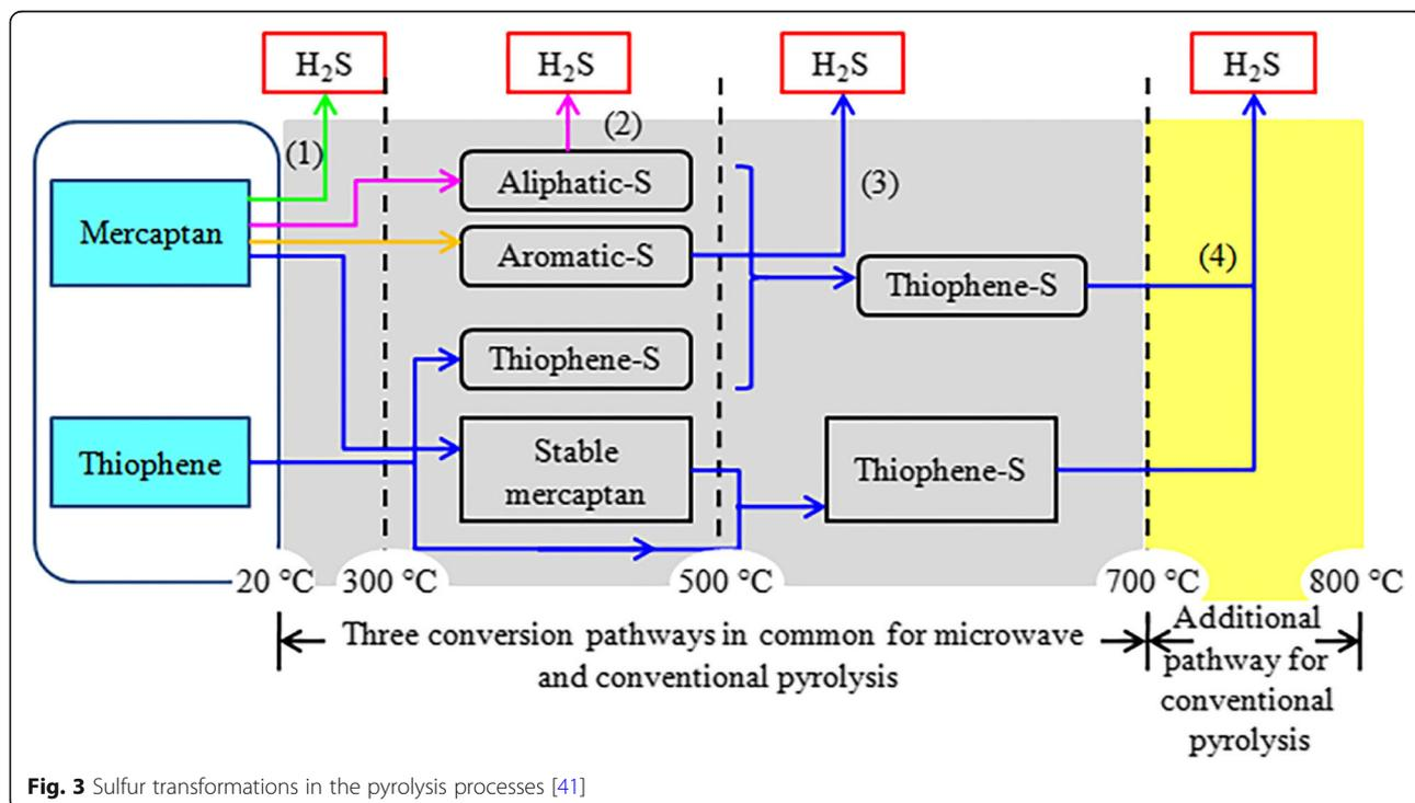
Fig. 3 Sulfur transformations in the pyrolysis processes [41]
