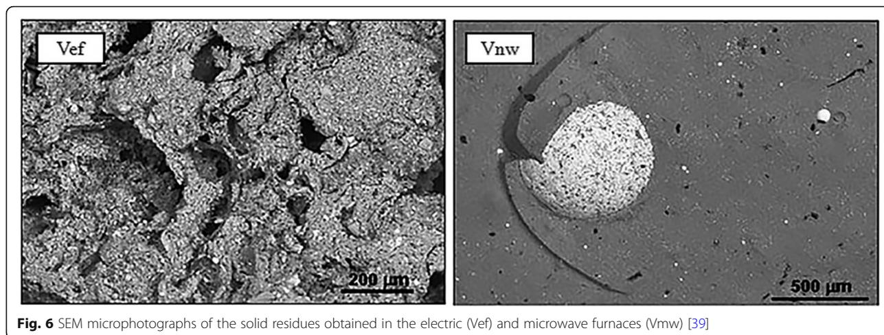
**Fig. 6** SEM microphotographs of the solid residues obtained in the electric (Vef) and microwave furnaces (Vnw) [39]
