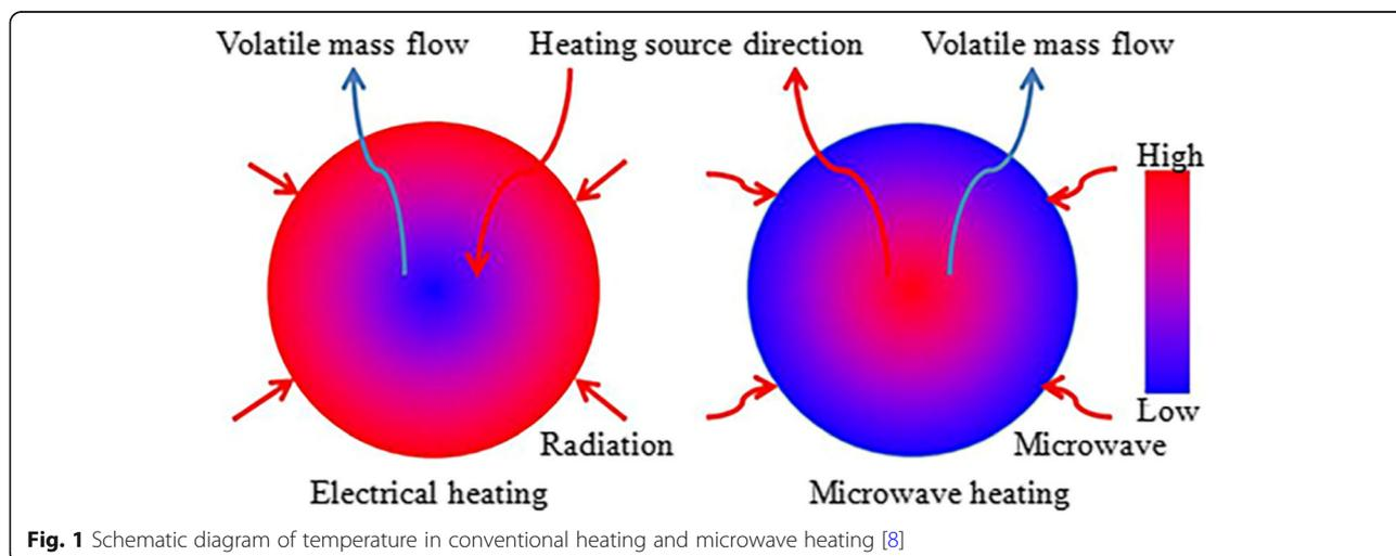
Fig. 1 Schematic diagram of temperature in conventional heating and microwave heating [8]
