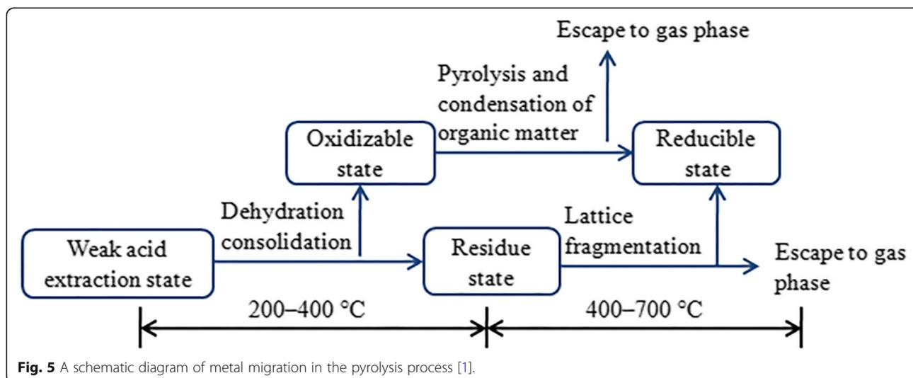
**Fig. 5** A schematic diagram of metal migration in the pyrolysis process [1].
