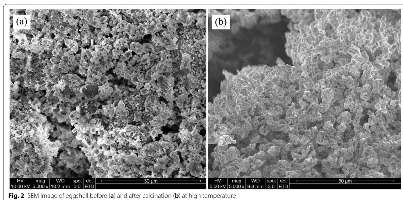
**Fig. 2** SEM image of eggshell before (a) and after calcination (b) at high temperature
