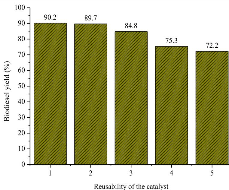
**Fig. 4** Reusability of the WES derived catalyst (CaO-based catalyst). Conditions: MTOMR 9:1; catalyst loading 5 wt%; reaction time 165 min; 65 °C; microwave power of 800 W
