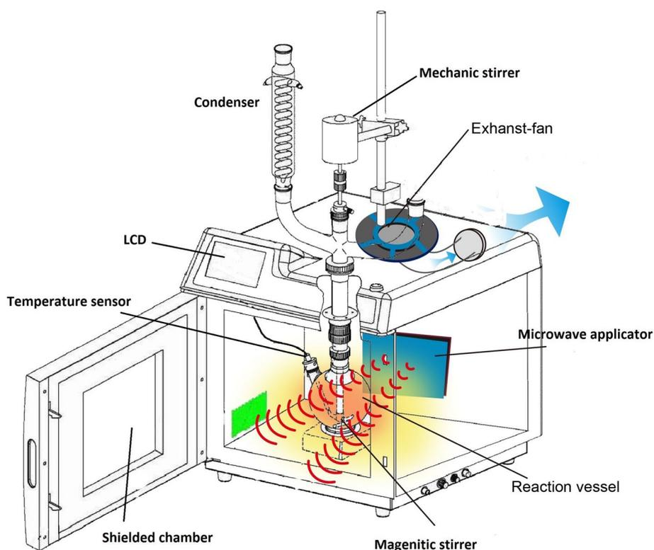
**Fig. 1** Schematic diagram of the experimental setup (microwave system structure). (Reprinted with permission from Lin et al. [5]). Copyright (2020), Elsevier [License Number: 5270740247480]
