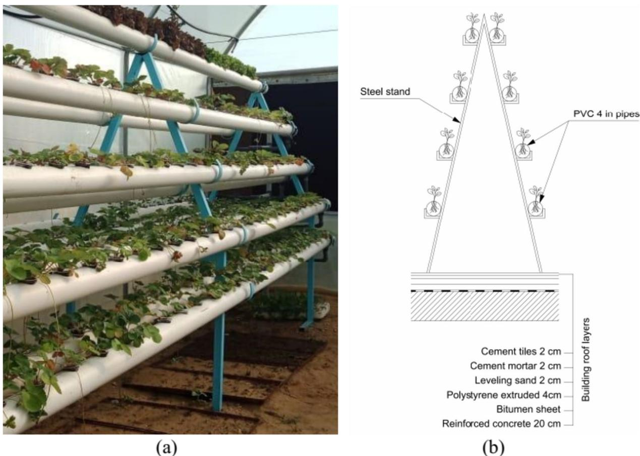
**Fig. 8** a The NFT green roof system [26], b Illustrative cross section for NFT (authors)
