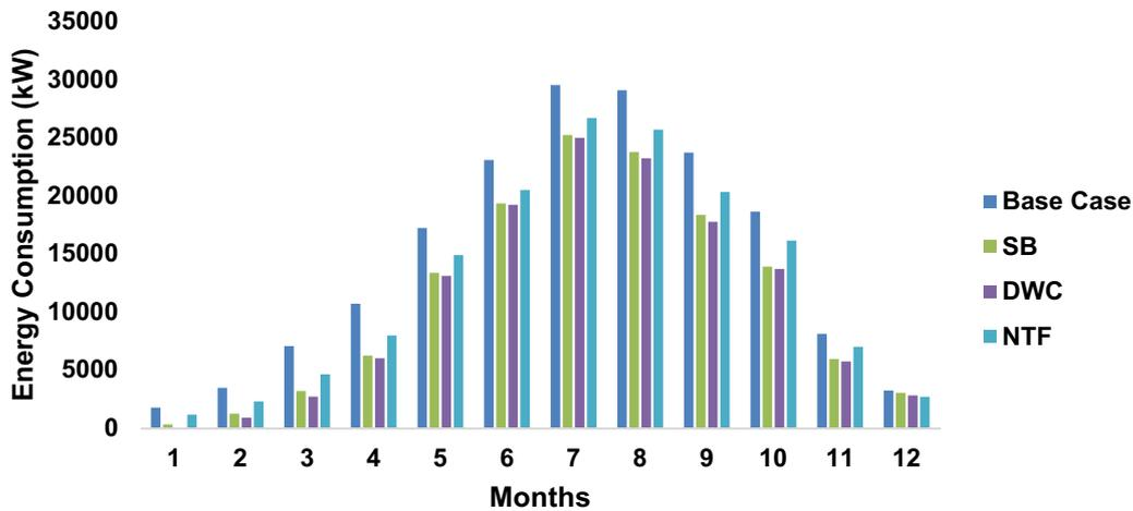
Fig. 11 The annual energy consumption for different systems
