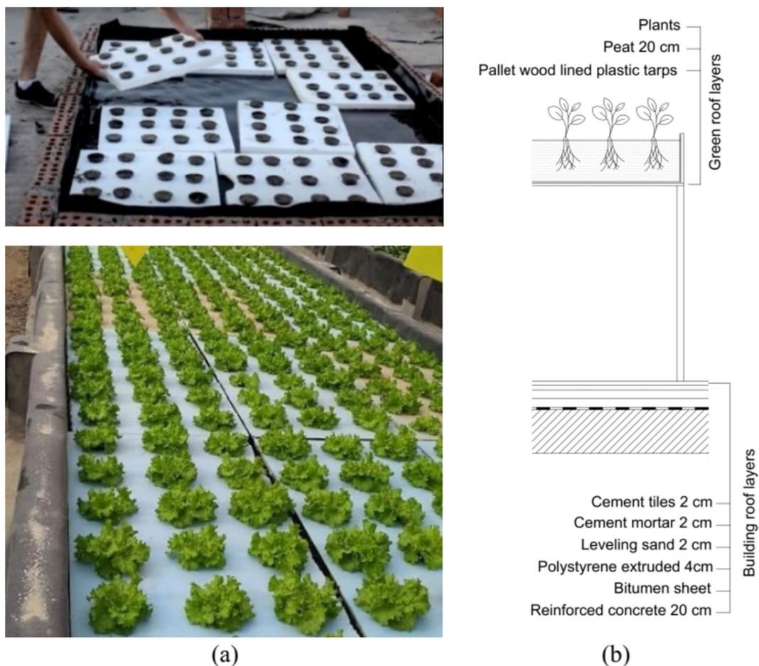
**Fig. 9** a The DWC green roof system [29], b Illustrative cross section for DWC (authors)
